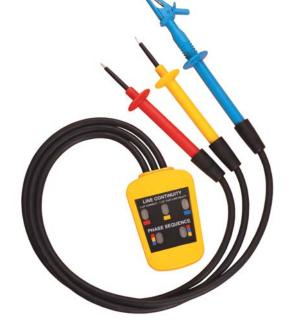
A fast, effective method of identifying worn or unmarked cables, and ensuring all 3-phase outlets and machinery are wired correctly. The PC15250 will also quickly and simply prove continuity of all three lines, or identify which are faulty as well as showing the sequence of phase rotation.
