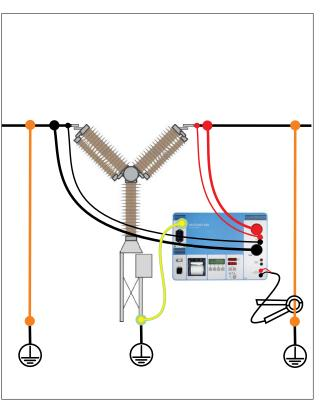
You can make tests with both sides of the test object grounded, an additional safety feature.
