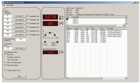
The Windows program makes it easy to manage/save all test results in a simple way. All information, meta-data of the test object e.g. a circuit breaker and the test results are stored together and they can easily be transferred to Microsoft® Excel for further analysis.
