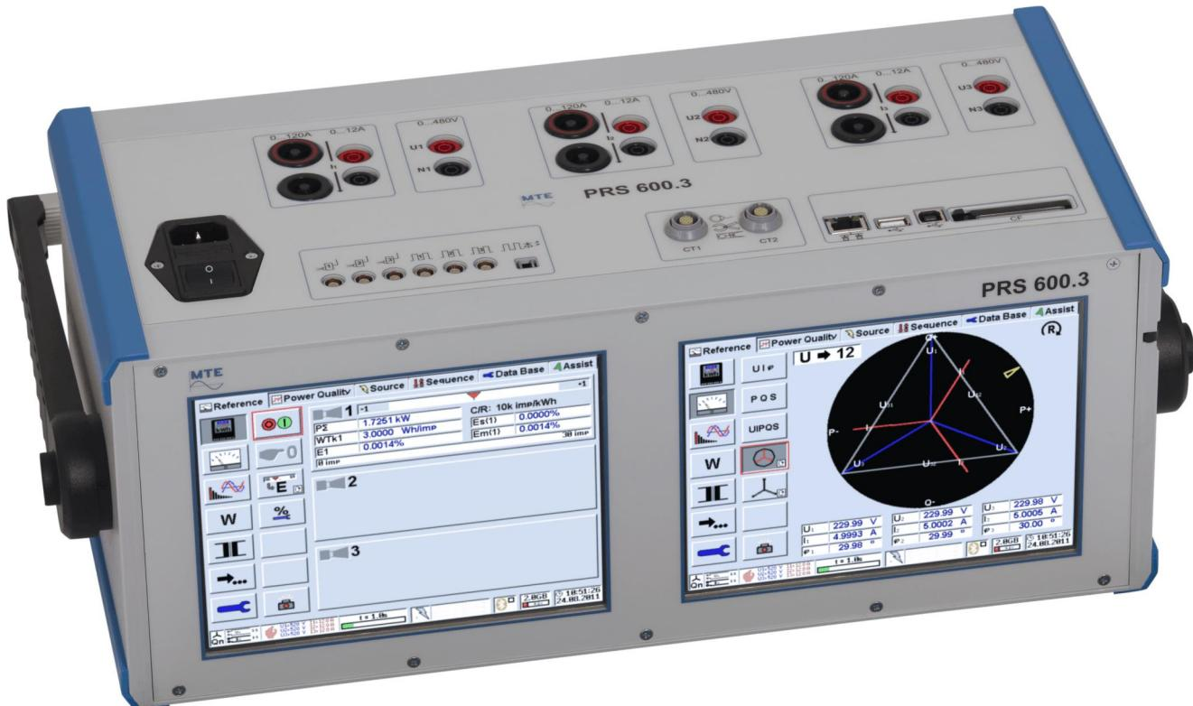
The PRS 600.3 is a combination of a three-phase Portable Reference Standard of class 0.02% and an IEC 61000-4-30 Class A compatible Power Quality Analyzer with 3 voltage and 3 current channels. The device is equipped with two 8.4" colors TFT displays based on touch screen operation. The Reference Standard is used to test single and three phase meters, instrument transformers and installations on site.
