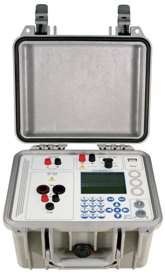
The CheckSystem 2.1 portable test system consists of an integrated single-phase current source and a single-phase electronic reference standard of accuracy class 0.2. Characteristic features of the CheckSystem 2.1 are its wide measuring range, high accuracy and high tolerance to unwanted external influences.
