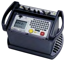
DLRO600 measures resistances between 0.1 \mu\Omega and 1 \Omega , at high currents. It can provide test currents from 10 amps up to 600 amps subject to the load resistance and supply voltage. It is ideal for testing busbars.
