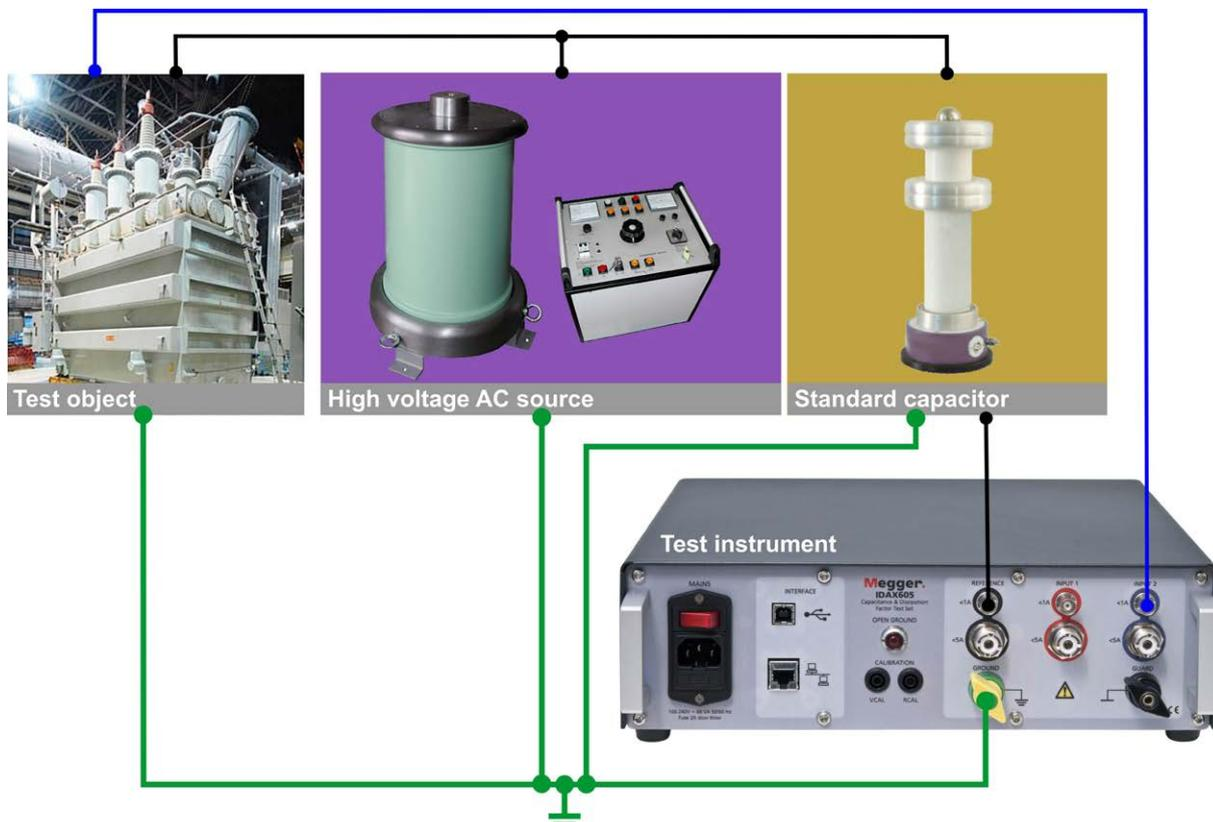
CDAX605 together with a high voltage AC source and a standard capacitor forms a complete setup for insulation testing.
