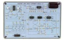
Variable duty ratio oscillator. RS, T, D, JK flip flop. Preset left/right shift register circuit. Noise elimination circuit.
