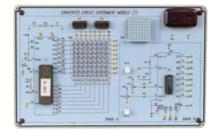
Construction dynamic scanning counter with single chip microprocessor. 8- bit converter circuit.
