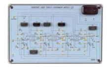
JK flip flop: asynchronous/synchronous, binaries up/ down bi-directional counters. Ring counter circuit, Johnson's counter circuit.
