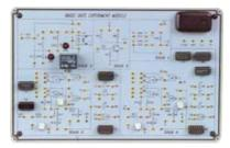
NOR NAND gate circuits, XOR gate circuits, comparator circuit experiments, Schmitt gate circuit, open collector gate circuits.
