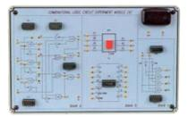
4 to 2 bit encoder. 4 to 2 bit decoder. Decoder circuit experiments (decoding 7-segment display with BCD code).
