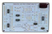
10 to 4 bit encoder. Multiplexer circuit experiments. Digitally controlled analog multiplexer/demultiplexer circuits. Bi-directional transmission with CMOS IC.
