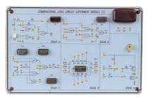
Three-state gate circuit. Adder. Arithmetic logic unit. Bit parity generator.
