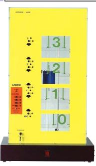
The ASC89 lift is a model which may be connected to a PLC or some microprocessors.
