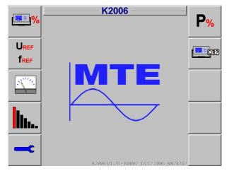
The main functions, error %, test against U-ref, f-ref, load values  $\text{UI}\phi$ , harmonics and basic system settings are directly accessed with soft keys.
